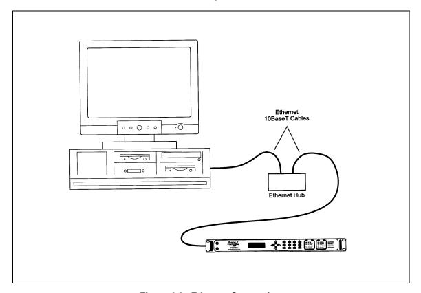
Figure 4-3. Ethernet Connection
