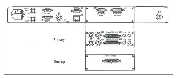
Figure 5-1. SFC Upconverter Back Panel
