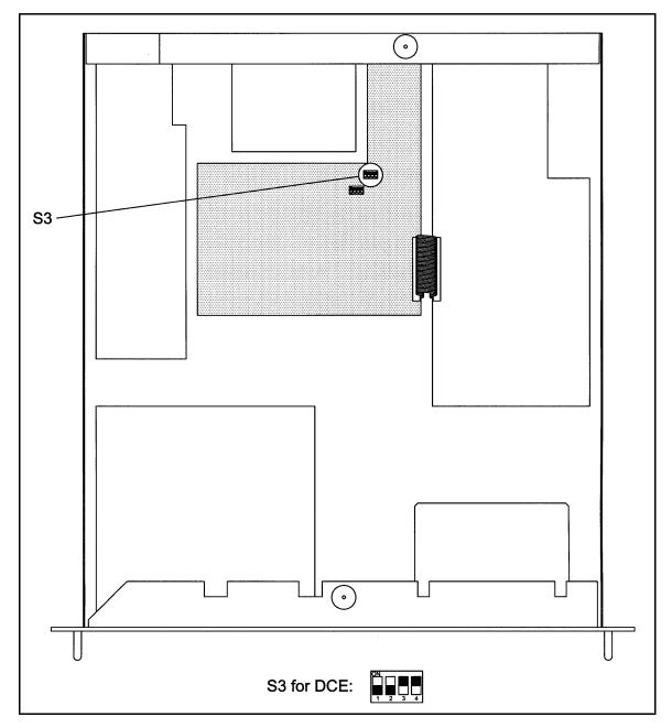
Figure 5-2. DIP Switch Settings for DCE
