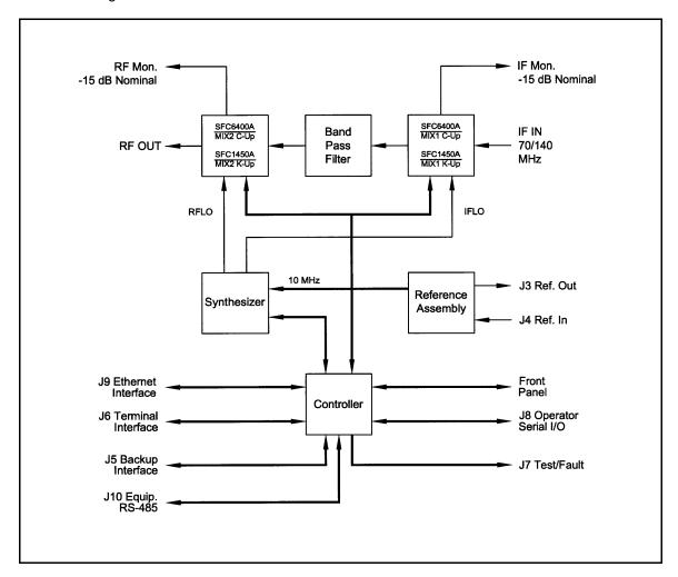
Figure 3-1. SFC Upconverter Block Diagram
