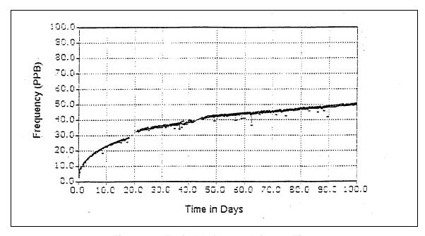
Figure 4-2. Typical Reference Aging vs. Time
