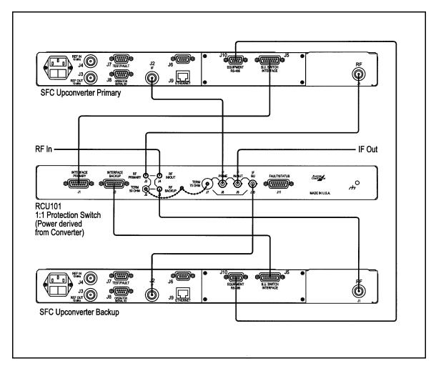
Figure 3-2. RCU101 Typical Interconnection with SFC Upconverters
